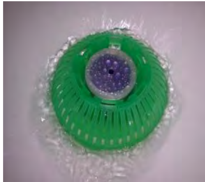
Figure 1: Picture showing the water level during flushing test.
