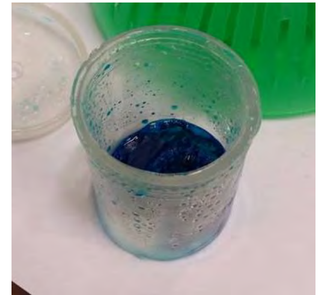
Figure 2: Picture showing test sample after 12,500 cycles of high pressure flushing.
